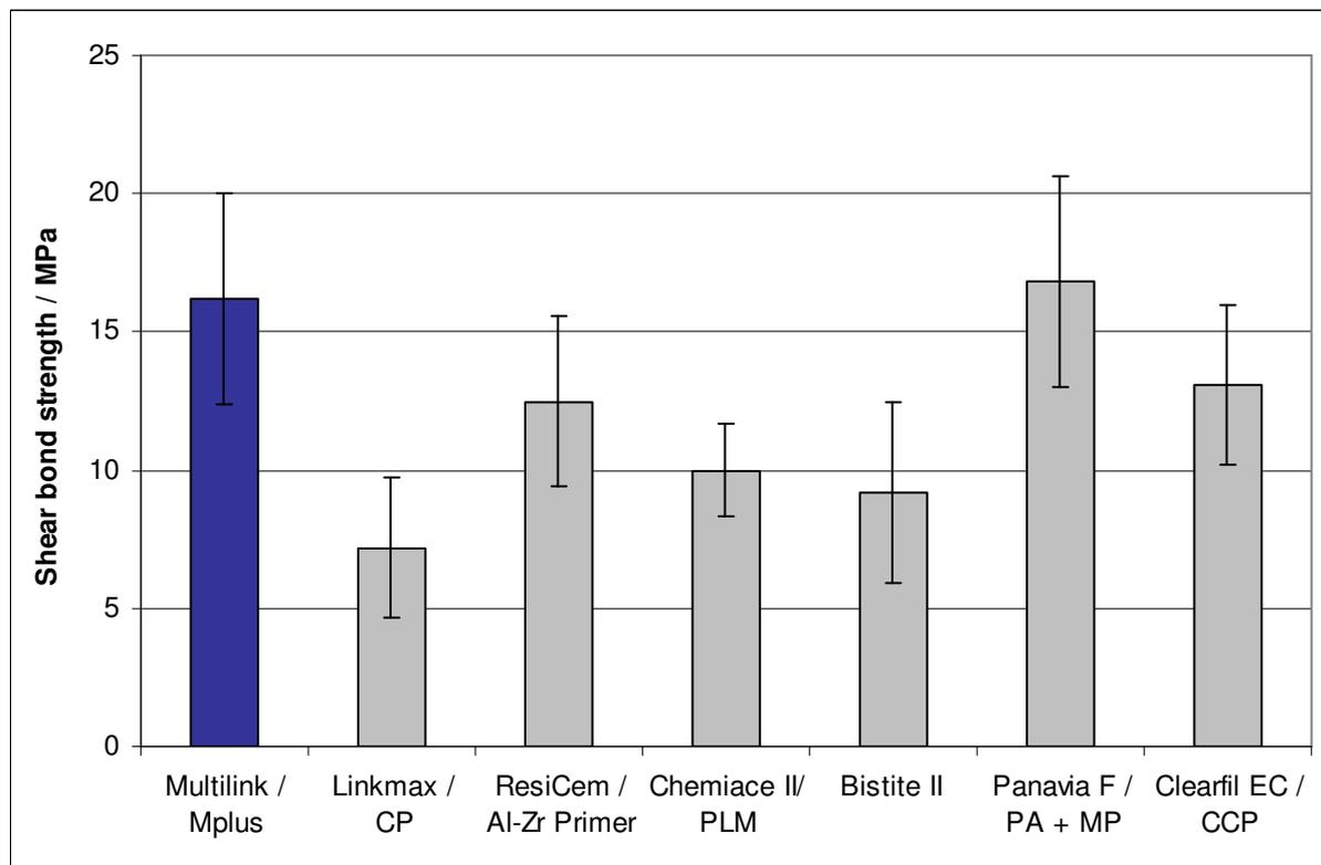
Fig. 4: Shear bond strength of Multilink Automix in the presence of Monobond Plus on the zirconium oxide material Lava. Tested systems: Multilink Automix/Monobond Plus (Ivoclar Vivadent), Linkmax/Ceramic Primer (GC), ResiCem/Al-Zr Primer (Shofu), Chemicace II/Porcelain Liner M (Sun Medical), Bistite II (Tokuyama Dental), Panavia F 2.0/Porcelain Activator/Mega Primer (Kuraray Medical) and Clearfil Esthetic Cement/Clearfil Ceramic Primer (Kuraray Medical) (Prof. Irie, Tokyo, 2008).
