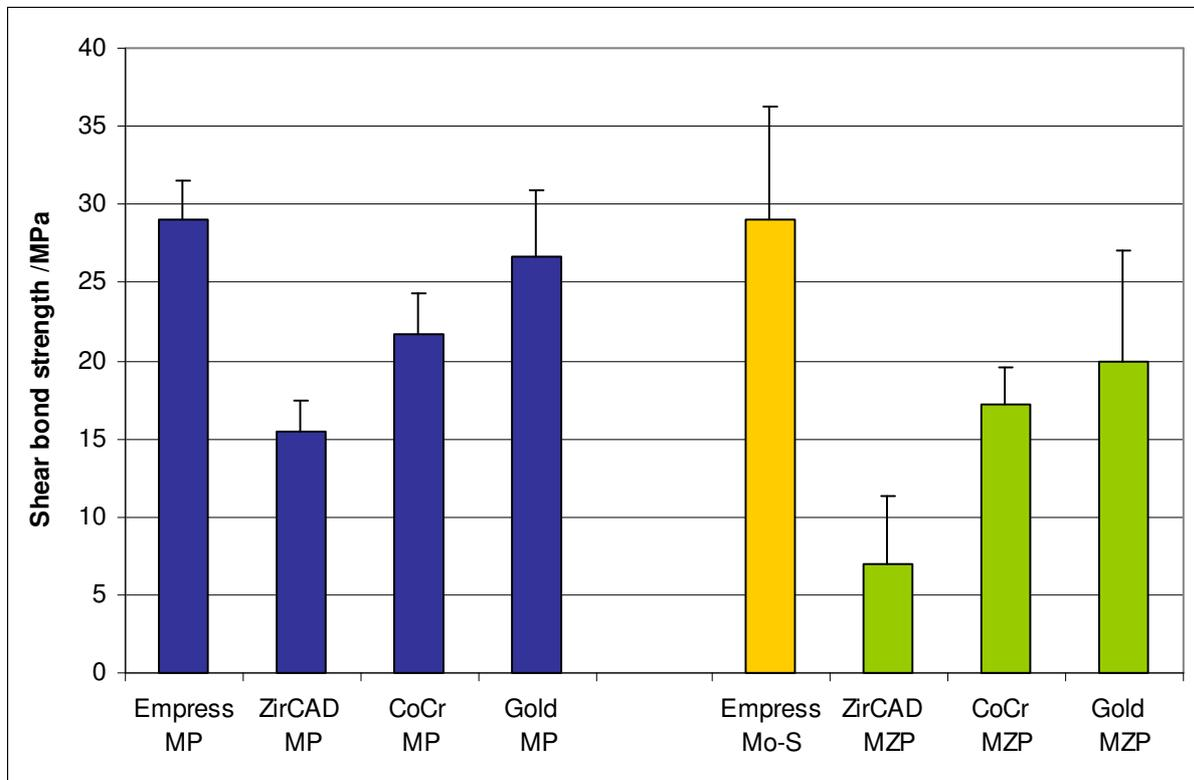
Fig. 3: Shear bond strength of Monobond Plus (MP) in comparison with Monobond-S (Mo-S) and Metal/Zirconia Primer (MZP) on IPS Empress, IPS e.max ZirCAD, chromium-cobalt alloy and high-gold alloy (Prof. Powers, Dental Advisor, 2008)
