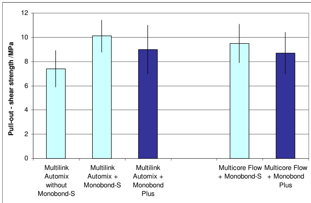
Fig. 5: Pull-out tests with FRC Postec Plus following adhesive cementation in the presence of Monobond-S or Monobond Plus (Ivoclar Vivadent, R&D 2008)
