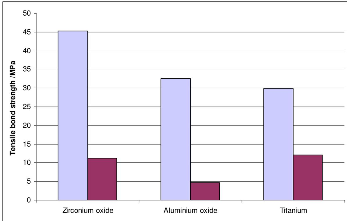
*Fig. 1: Tensile bond strength achieved with Monobond Plus and Multilink Automix without (light) and after (dark) pre-treatment with phosphoric acid (Ivoclar Vivadent, R&D 2008)*
