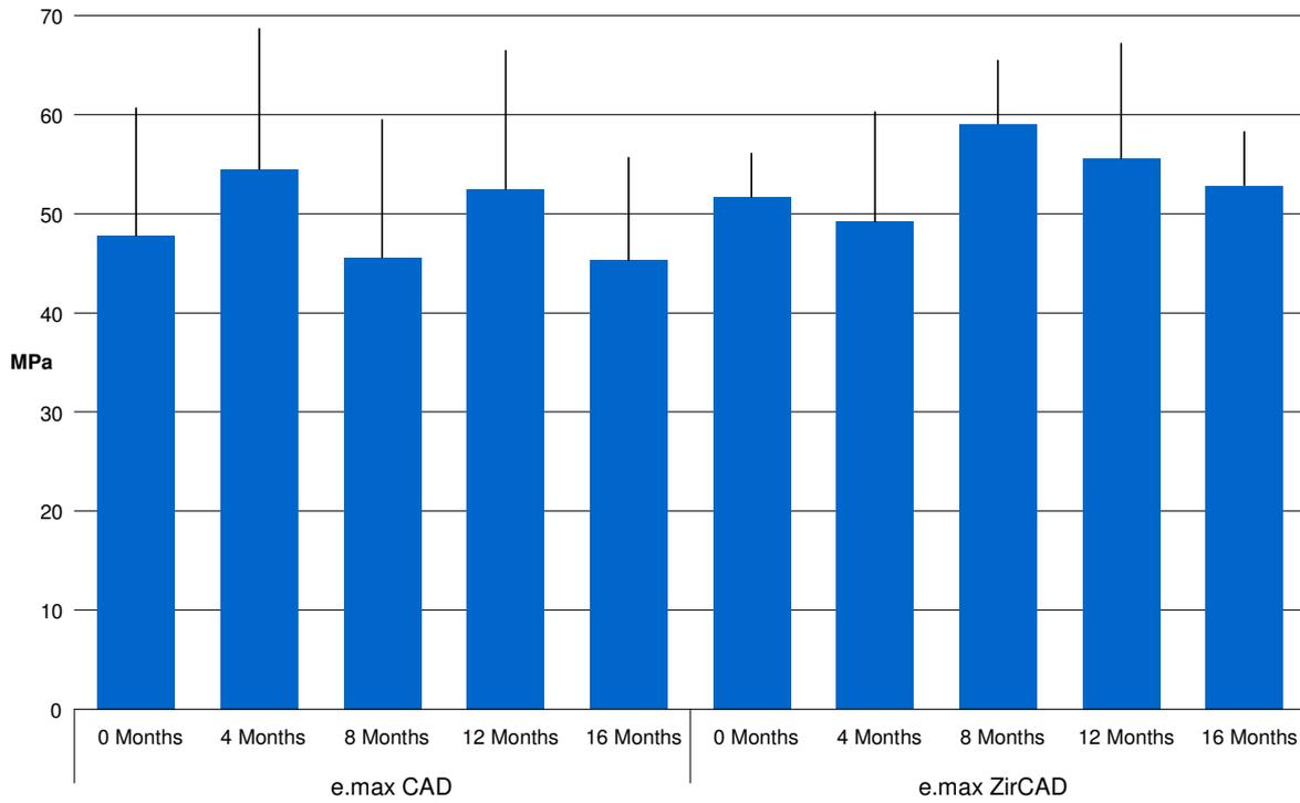
Fig. 6: Tensile strength values on IPS e.max CAD and IPS e.max ZirCAD following luting with Multilink Automix and Monobond Plus after storage at room temperature (Ivoclar Vivadent R&D, 2010)
