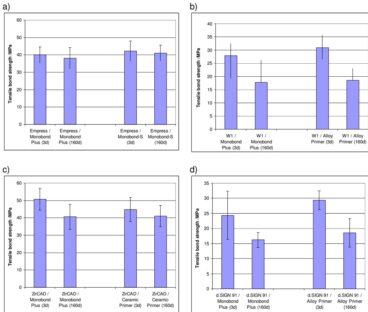
Fig. 2: Tensile bond strength of Monobond Plus on different substrates in comparison with Monobond-S, Ceramic Primer and Alloy Primer after 3 or 160 days of immersion in water: a) leucite glass-ceramic IPS Empress b) Pd-based alloy W1 c) Y-TZP IPS e.max ZirCAD d) gold alloy d.SIGN 91 (Prof. Kern, University of Kiel, 2008)
