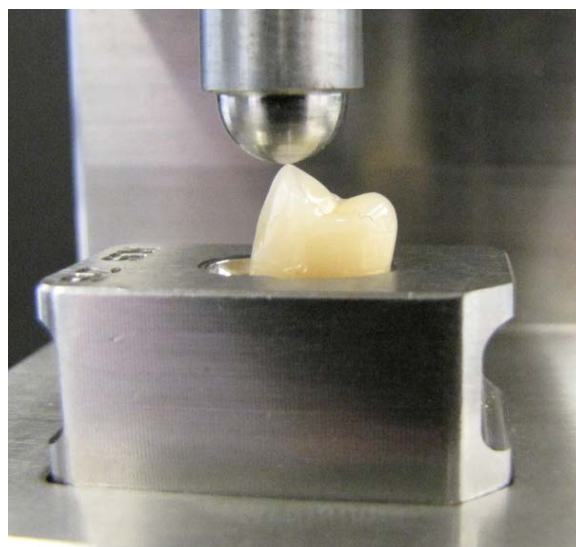
Fig. 11: Setup for chipping test.
